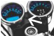
HAZARD SIGNAL BUTTON
