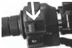
TURN SIGNAL SWITCH
